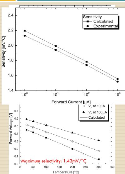
■ SBD forward biased at constant current  $V_F(T) = n\varphi_{Bn} - [n\varphi_{Bn} - V_F(T_0)] \frac{T}{T_0}$ ■ Sensor detection selectivity  $S = \frac{n\varphi_{Bn} - V_F(T_0)}{T_0}$ ■ High  $n\Phi_{Bn}$  - high selectivity
